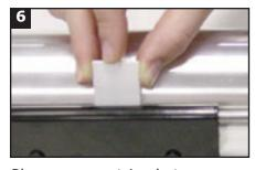
Place spacer strips between roller drum and resistance unit to achieve appropriate spacing. **Note:** Roller resistance unit is shipped in resistance level 5. This has the closest gap to the roller drum. The spacing setup should be completed in this setting to prevent the drum from contacting the resistance unit during use.
